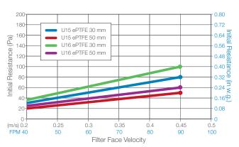
Recommended final resistance: 500 Pa. Maximum operating temperature: 70 °C. Fire classification: UL 900. See complete marking on product. Performance graph: MEGAcel II ME 610 x 1220 x 69 mm (HxWxD)
